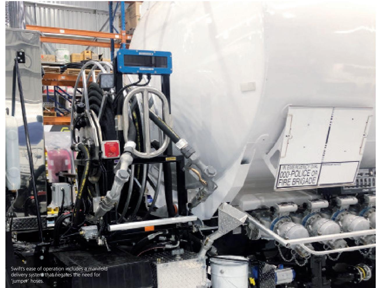
arrangement ensures there is no need to switch or ‘jump’ hoses between compartments – an operation which used to inevitably result in a small amount of fuel leaking onto the ground.
